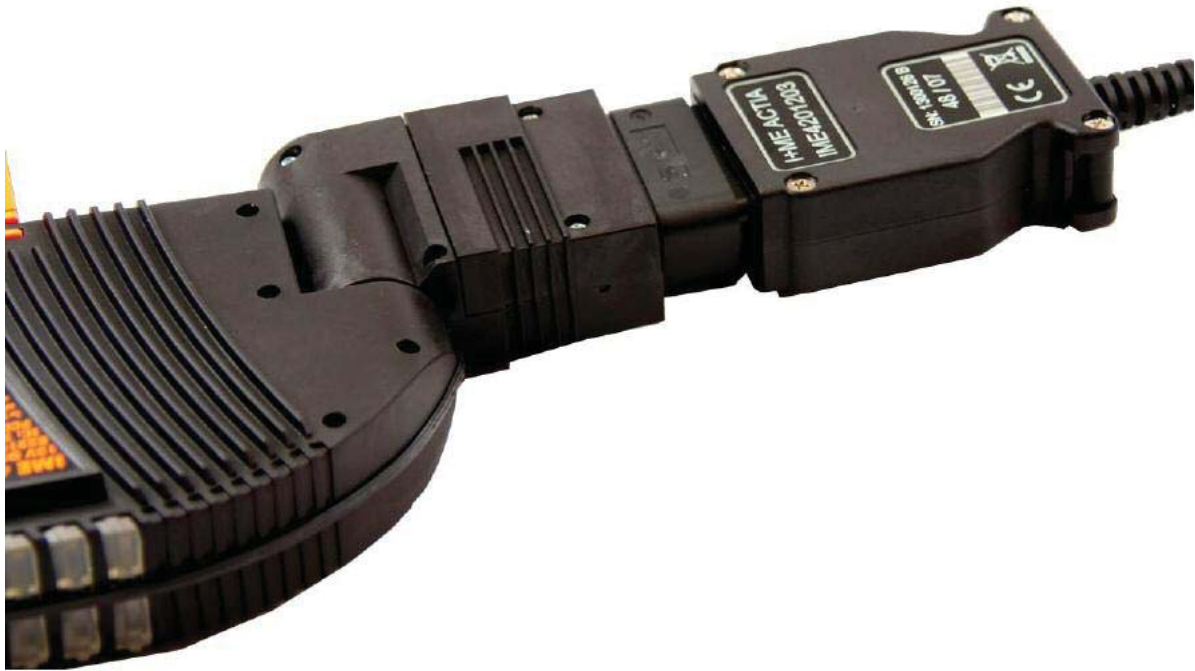
Connection of ICOM A with ICOM C
